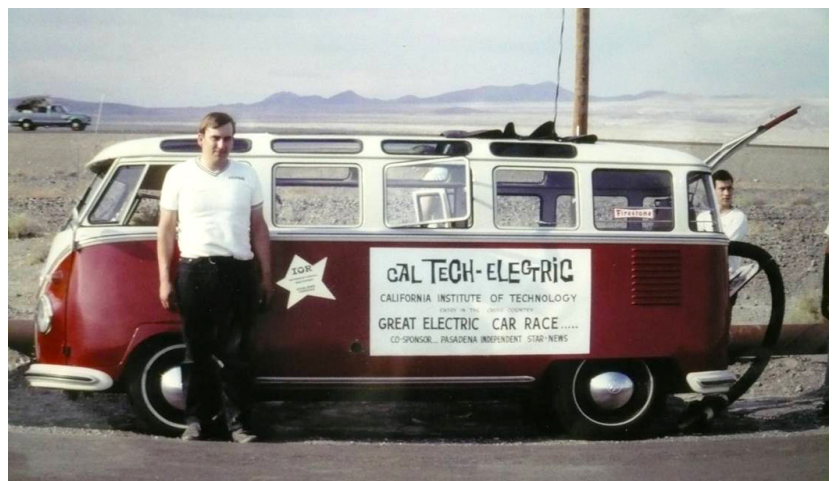
Wally Rippel and his Volkswagen bus, converted to a fully electric vehicle for the cross country race against MIT
